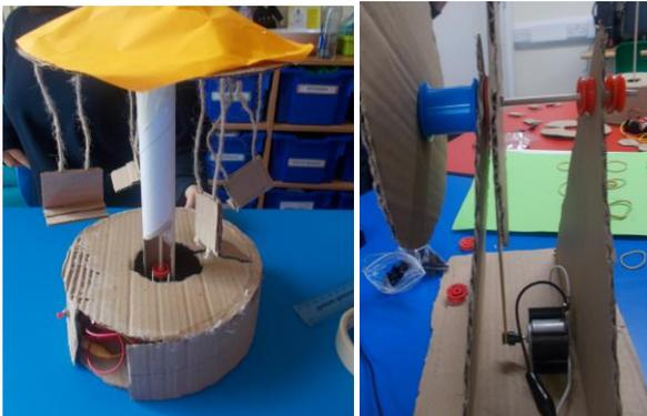
A student completed a design of a lighthouse. He used a circuit with a switch to control the light on top of the lighthouse which was used as a signal.
